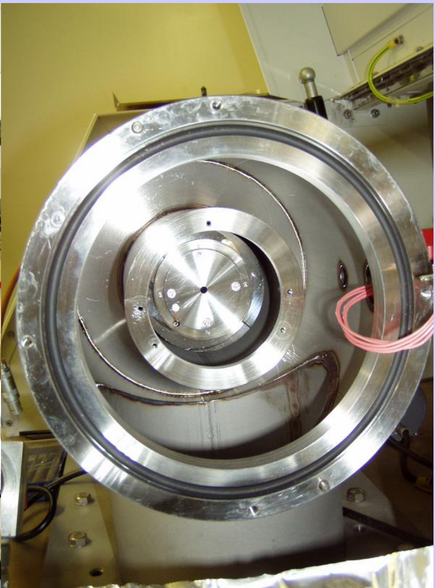
View of Lens Stack in High Vacuum Chamber of VG-PQ2S
